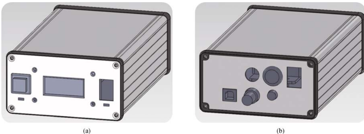
Fig. 10 3D rendered Solidworks model of pulsed high voltage modulator prototype
